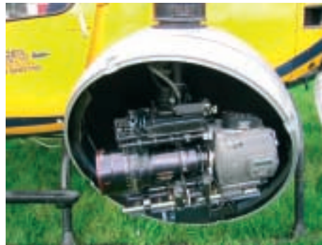
The Wescam F435 configured with Panavision Genesis on set for His Dark Materials: Golden Compass
